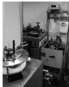
Fig. 2. Helium gas recovery system
