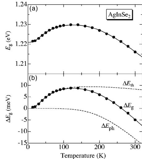
FIG. 2. (a) Plots of  $E_g$  vs  $T$  for AgInSe<sub>2</sub> determined from the optical absorption measurements. The solid line represents the least-squares fit of the experimental  $E_g(T)$  data to Eq. (3). (b) Plots of  $\Delta E_g$  vs  $T$  for AgInSe<sub>2</sub>, together with those for  $\Delta E_{th}$  and  $\Delta E_{ph}$  calculated from Eqs. (4) and (9), respectively. The solid circles represent the experimental data.
