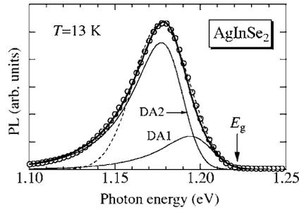
FIG. 6. Theoretical fit of the PL spectrum for  $\text{AgInSe}_2$  measured at  $T = 13$  K. The dashed line represents the DA-pair emissions obtained from Eq. (10), while the heavy solid line shows those from Eq. (13). The light solid lines represent the deconvolution of the heavy solid line into two individual peaks (DA1 and DA2). The vertical arrow indicates the position of the bandgap energy at  $T = 13$  K.
