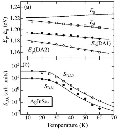
FIG. 7. (a) Variations of the band-gap energy  $E_g$ , "demarcation level" width  $E_d$ , and DA-pair peak energies  $E_p$ 's as a function of temperature  $T$  for AgInSe<sub>2</sub>. (b) Variations of the strength parameters  $S_{\text{DA1}}$  and  $S_{\text{DA2}}$  as a function of temperature  $T$  for AgInSe<sub>2</sub>. The solid lines show the calculated results of Eq. (14).
