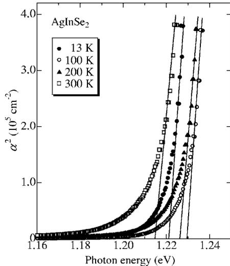
FIG. 1. Plots of the square of the absorption coefficient  $\alpha^2$  vs photon energy for AgInSe<sub>2</sub> at  $T=13$ –300 K. The intercept point on the energy axis gives the band-gap energy  $E_g$  at each temperature.
