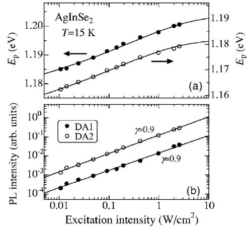
FIG. 8. (a) Excitation intensity dependence of the PL peak energies  $E_p$ 's and (b) integrated PL intensities for the DA1 and DA2 emissions in AgInSe<sub>2</sub> at  $T = 15$  K. The solid lines in (a) and (b) are calculated from Eqs. (16) and (17), respectively.
